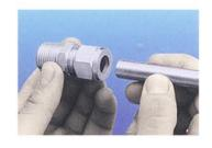
Make a mark at the 'O' position. Now tighten the nut 1-1/4 turns for the final assembly to be finished. The tube is sealed securely on the bottom and the ferrule has swaged onto the tube.
